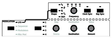
Mopho has four low frequency oscillators (LFOs). The LFOs can be freerunning, synced to keystrokes, or synced to the sequencer and MIDI clock. To edit the LFO parameters, choose LFO in the Modulation section.
