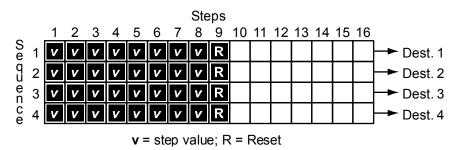
**Tip:** Using Reset while programming a sequence can be helpful. For example, when programming a specific melodic line, start by shortening the sequence to four or eight steps until those steps are set, and then gradually move the reset point to lengthen the loop until the desired number of steps is playing.
