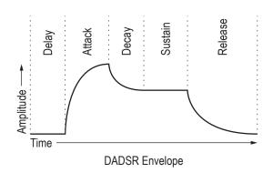
**Repeat:** Off, On—When on, the Delay, Attack, and Decay segments of the envelope repeat. Sustain still affects the level at which the Decay segment ends, but—instead of sustaining at a fixed level while a note is gated on—Delay, Attack, and Decay loop until the note is turned off. The Release segment begins when the note is gated off, just as it does when Repeat is off. See the illustration on the following page.
