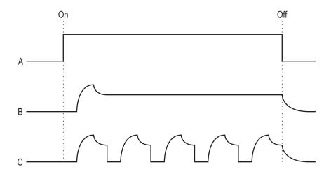
A: The gate generated by pressing, holding, and then releasing a key.
