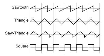
**Pulse Width:** 0...99—Sets the pulse width or *duty cycle* of the square wave. A value of 50 results in a true square wave with equal alternating high and low levels. Increasing or decreasing the value from 50 causes the waveshape to become asymetrical. Lower values narrow the postive-going portion of the
