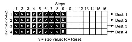
**Tip:** Using Reset while programming a sequence can be helpful. For example, when programming a specific melodic line, start by shortening the sequence to four or eight steps until those steps are set, and then gradually move the reset point to lengthen the loop until the desired number of steps is playing.
