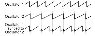
**Tip:** Try routing an envelope or the mod wheel to oscillator 1 frequency for the familiar sync sweep sound.
