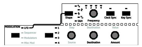
Mopho x4 has four low frequency oscillators (LFOs) per voice. The LFOs can be free-running, synced to keystrokes, or synced to the sequencer and MIDI clock. To edit the LFO parameters, choose LFO in the Modulation section.
