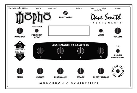
Input Gain — Used to adjust the gain of AUDIO IN. For more about using Mopho to process external audio, see page 11. For low-level sources (like guitars), INPUT GAIN should be turned up. For line-level sources, it will usually be turned down. Turning it down does not turn it off, it just decreases the gain. External Input Volume (see *Mixer Parameters* on page 17) controls the amount of signal that gets mixed into the filter and must be turned up for any audio—external or feedback—to be heard.
